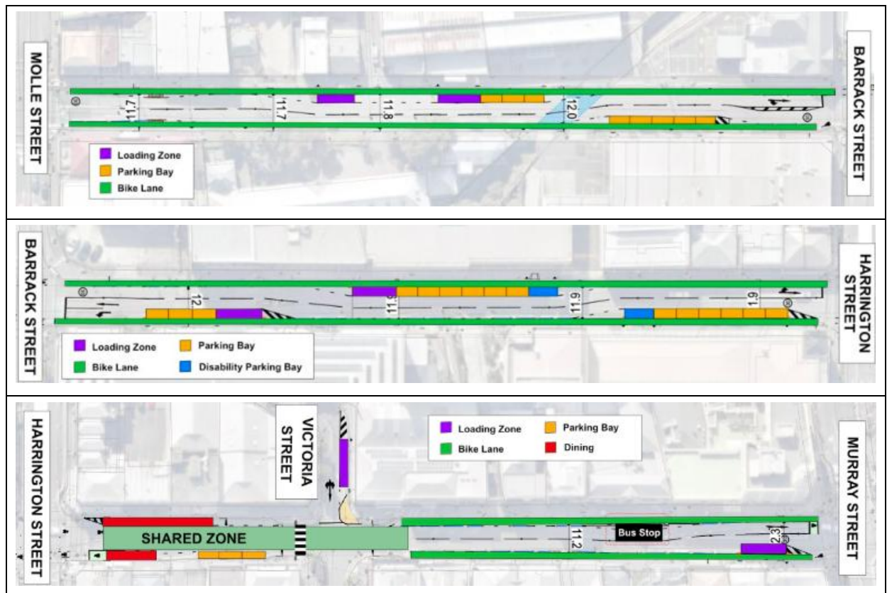
Figure 6 On-Road Bicycle Lane Design
